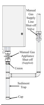
**A** WARNING: Never use an open flame to test for gas leaks, as property damage, personal injury, or death could result.
